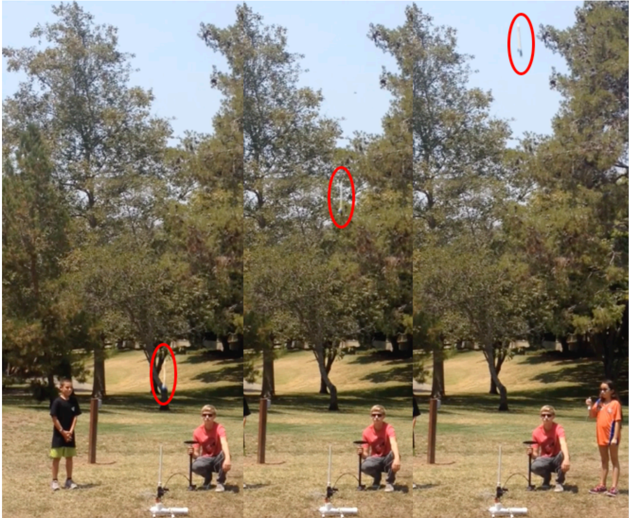
Figure 1, Three consecutive frames of a rocket launch at 30 frames per second. Red circle identifies rocket position.
