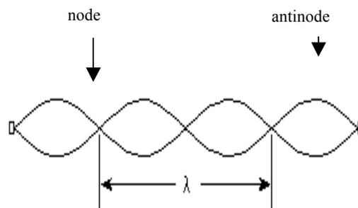
Figure 2. Example of a Standing Wave Pattern
