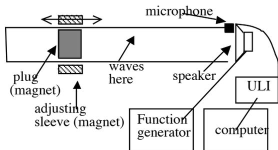
Figure 1. Schematic for Standing Sound Waves Experiment
