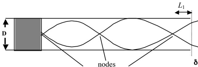
Figure 3. The Standing Wave in the Tube
