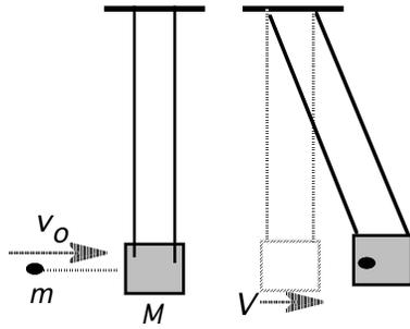
Suppose a bullet ( $m$ ) is fired horizontally (initial speed  $v_o$ ) into a block ( $M$ ) which is suspended from strings of length  $L$ , as shown.
