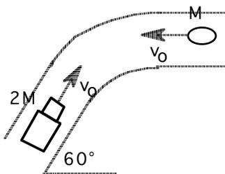
Consider a that car traveling west and a truck traveling  $60^\circ$  north of east collide, stick together, and slide to a stop. Assume the friction with the pavement has no effect on the collision itself.
