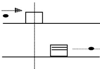
Suppose a bullet is fired at a block on a horizontal frictionless surface. The mass of the bullet is  $m$  and the mass of the block is  $M=10m$ . If the bullet has an initial speed of  $v_o$ , passes through the block and emerges with speed  $v_f=v_o/10$ , determine the final speed of the block.
