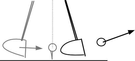
Suppose a golf ball is struck by a golf club. Assume that the collision is elastic. If the ball has a mass of 50 g and the golf club head has a mass of 200 g, determine the ratio of the launch speed of the ball to the clubhead speed just before contact. [Make the simplifying assumption that it is a one-dimensional collision in which momentum is conserved.]
