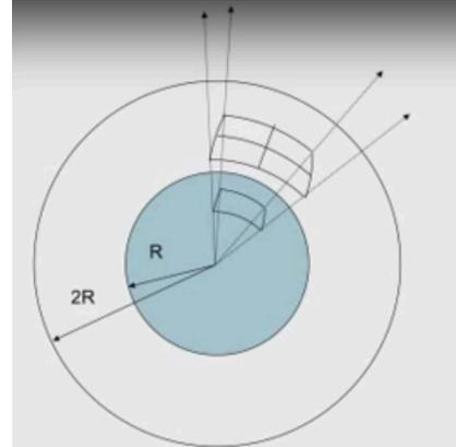
Fig.1 Light propagates equally in all directions from a point source in the middle. The flux of power that escapes through the smaller sphere must also pass through the larger sphere. Because the same flux is spread over a larger surface at the larger sphere, the intensity of light is weaker at the larger distance.
