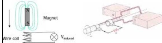
Magnets used to generate voltage and current
