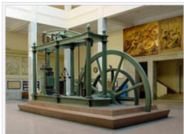
A Watt steam engine. James Watt transformed the steam engine from a reciprocating motion that was used for pumping to a rotating motion suited to industrial applications. Watt and others significantly improved the efficiency of the steam engine.
