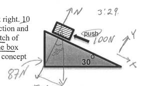
3. (15 pts) Your job is to keep boxes moving up a 30° incline as shown at right. 10 kg boxes are pushed from below on a surface with a 0.3 coefficient of friction and reach you with a speed of 3 m/s. You push the boxes up the next 4 m stretch of ramp with a force of 100 N as shown, and we want to find the speed of the box when you're done pushing it. Clearly show your work, identifying which concept you're using.
