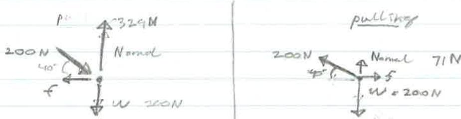
Since  $F = \mu N$ , the diagram with the smaller Normal force, pulling the mower reduces the normal force since some of it is taken away by the vertical component of your pull, giving a smaller frictional force. To get the same acceleration/work done, pulling the mower will minimize the force necessary.
