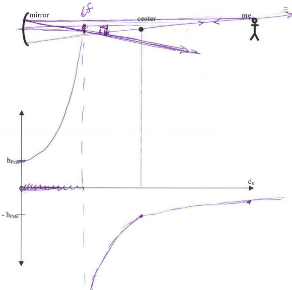
b) On the X-axis, mark where the image is a virtual image, by darkening that part of the X-axis.
