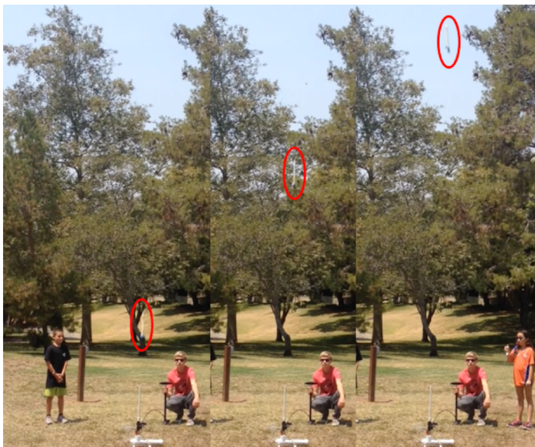
Figure 5: Three consecutive frames of a rocket launch at 30 frames per second. Red circle identifies rocket position
