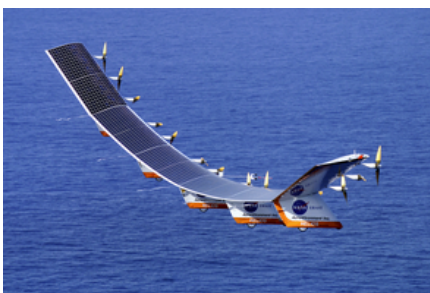
Figure 4: Solar energy is converted into electrical energy by solar cells, which is used to run a motor in this solar-power aircraft. (credit: NASA)
