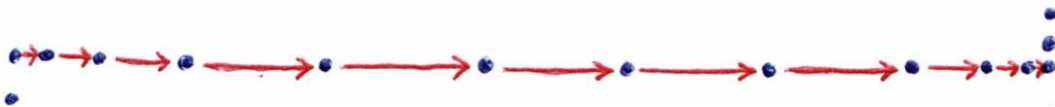
Figure 1.7 Motion map of ThrustSST setting land speed record, including time before it started moving and after it stopped moving
