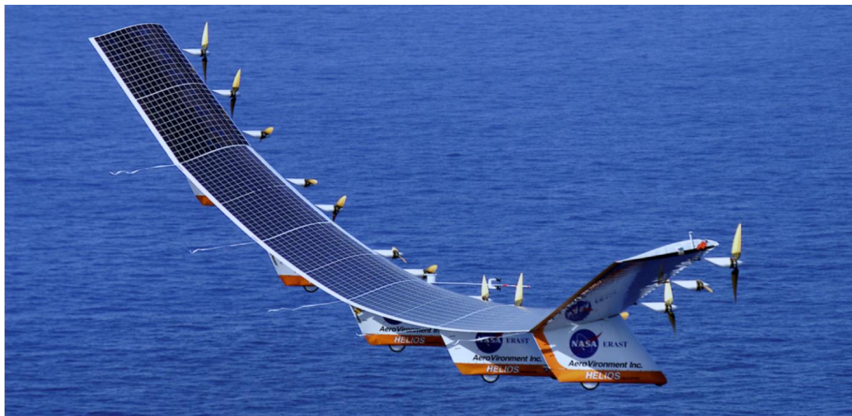
Figure 1.18 Solar energy is converted into electrical energy by solar cells, which is used to run motors in this solar-power aircraft. (credit: NASA)
