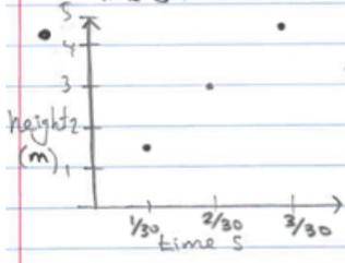
$\text{speed} = \frac{1.5 \text{ m}}{1/30 \text{ s}} = 45 \text{ m/s}$
