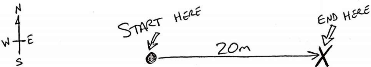
Figure 5.2: A displacement vector pointing East
