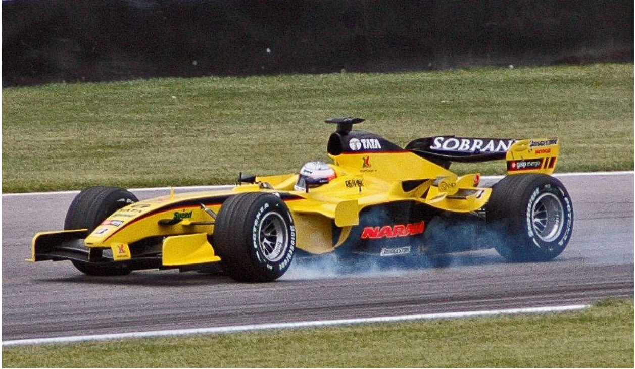
Figure 5.1 A racecar locking its brakes. The tires are smoking from the heat generated by friction with the road. (Photo credit: CC BY-SA 2.0, https://commons.wikimedia.org/w/index.php?curid=192252 )
