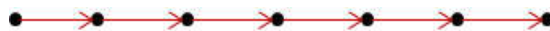
Figure 6.3 A motion map of a ball on a train moving at constant velocity
