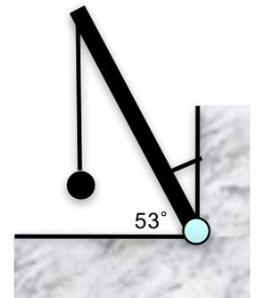
8. In the diagram at right, a string of some length supports a 100 kg ball. The length of the tilted rod is 10 m and the cable is attached 2.5 m from the pivot. From the drawing at right (make your own better drawing), estimate the tension on the cable and the force provided by the foundation at the pivot.
