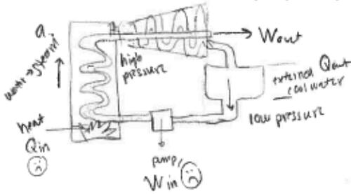
b. Rankine pumps water into a chamber where the water then turns into steam (volume expanded  $\sim 1000\times$ ). The steam then pushes the turbine blades to get work out. To turn steam back into water, there is an external cool water supply to lower the pressure & turn steam back into water that is then pumped again.
