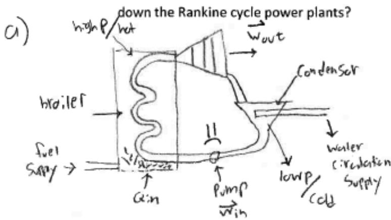
b) Cold water is pumped into a boiler where heat is being produced by some method (maybe a fuel is burned). Here the water is converted into steam which increases in ~~pressure~~ and volume, this steam escapes through a turbine and produces work out. The steam is then condensed back into water and the cycle repeats.
