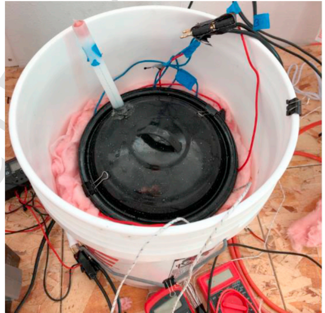
Fig. 4. Each solar panel powered a different heating technology in three insulated cook pots made of 4-quart steel pots insulated with pink fiberglass insulation around the perimeter and below (but not above), containing 3L of water.
