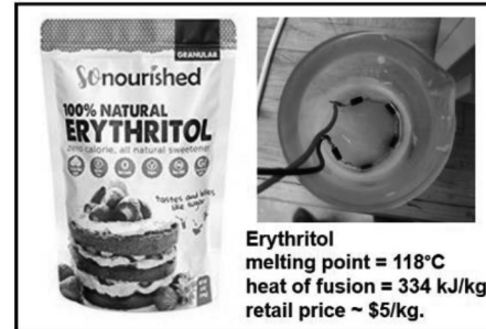
Figure 4. Erythritol, our Phase Change Material (PCM) is a readily available artificial sweetener (left), and is show partially melted in a diode chain (right).
