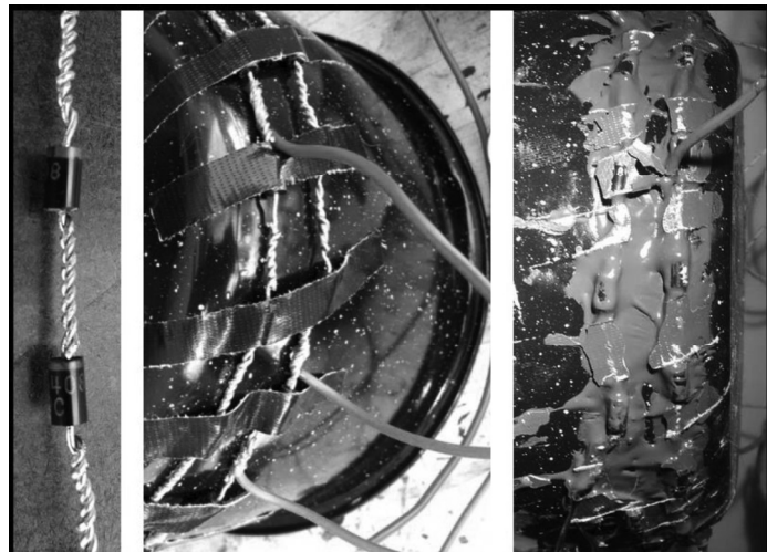
Figure 2. A diode chain is made by twisting diodes together (left), securing the chain to the bottom perimeter of a pot (middle), and gluing with a high-temperature glue (right).
