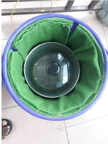
Figure 5. ISEC cooker in bucket with blankets epoxied to the inside.
