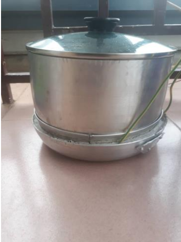
Figure 4. ISEC cooker with diode nest and metal cement-filled shield to protect diode chain.
