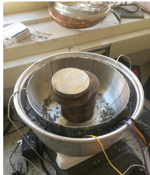
Figure 11. Diode nest inside container of molten erythritol with Aluminum shavings. Weights are added on top of the diode nest to keep it from floating too high while the erythritol solidifies. No insulation container is present in this photo.
