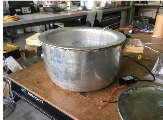
Figure 8. Initial design of PCTS cooker. The sides of the pot are filled with PCM.
