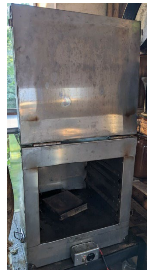
Oven ISEC, radiant heater
