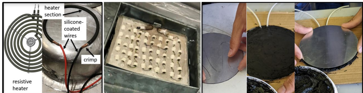
Resistive heaters can be made (from left) by cutting a section of an electrical cooking element and crimping the inner NiCr wire to power leads with copper tubing, threading NiCr wire through ceramic beads, and by sealing NiCr wire in furnace cement between aluminum sheets.
