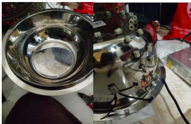
ISEC, resistive heater of NiCr wire through ceramic beads
