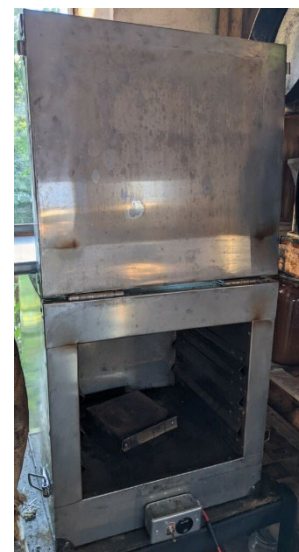
Oven ISEC, radiant heater
