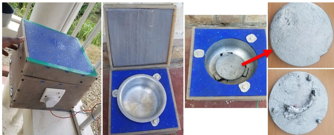
From left: recycled plastic housing, cook pot, heater plate, welded heating element under plate
