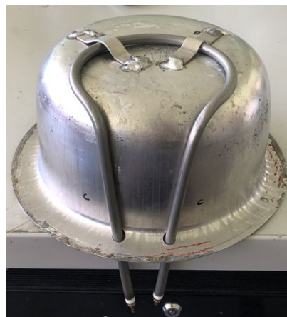
Immersion heater fit to inner cookpot
