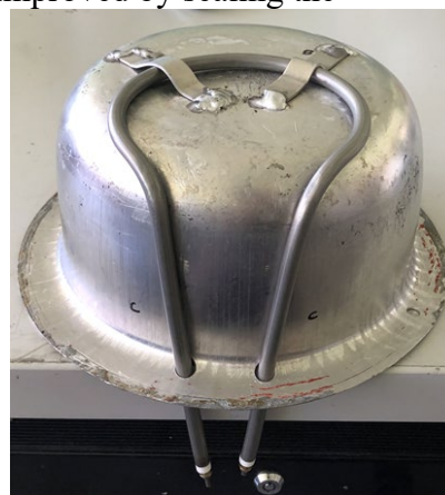
Immersion heater fit to inner cookpot
