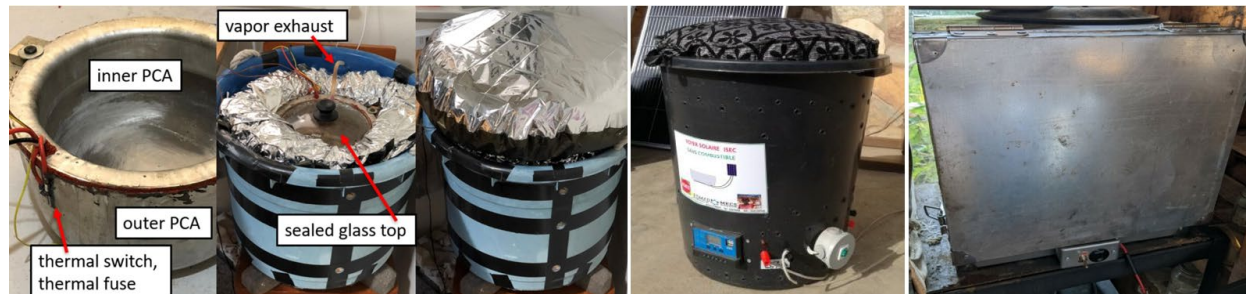
(left) Cylindrical ISEC with thermal storage, 3 (middle) Salma's direct connect ISEC, (right) LEF oven ISEC.
