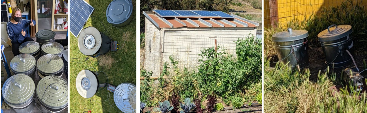
From left, Katarina with direct connect ISECs, testing outside the laboratory, mounted solar panels at the farm, and lithium titanate battery supplemented ISECs.
