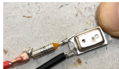
From left to right: Red power cable to copper tube clamp to thermal fuse to thermal switch.
