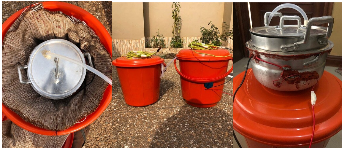
Fig. 9 Two ISECs with phase change material (erythritol) and wool insulation
