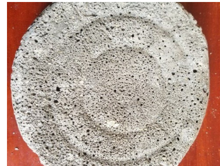
Rigid, insulating vermiculite concrete
