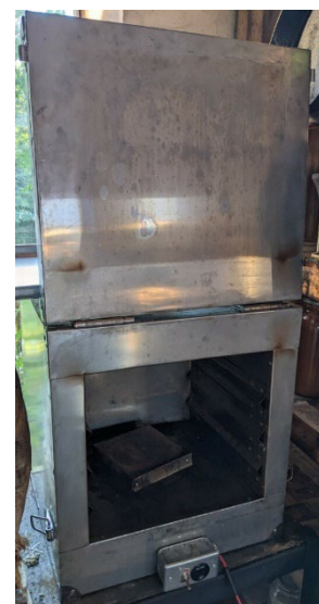
Oven ISEC, radiant heater
