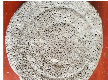
Rigid, insulating vermiculite concrete
