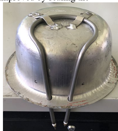
Immersion heater fit to inner cookpot
