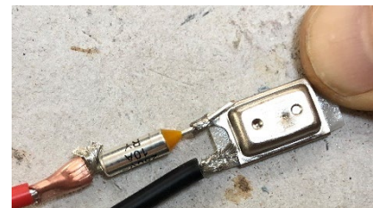
From left to right: Red power cable to copper tube clamp to thermal fuse to thermal switch.
