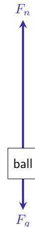
Figure 6.7: FBD of the ball when it is in contact with the ground, images 16 & 29 in Figure 6.5. Lengths of the arrows are not exact, but are intended to signify that F_g is the same as in Figure 6.6 and that F_n > F_g . [1]
