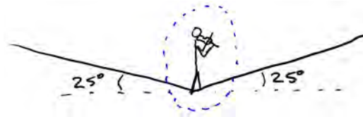
Figure 4.16: Sketch of the fiddler balancing on a rope. The blue dotted line indicates the "system" to be considered when making a free body diagram.[1]
