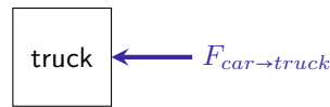
Figure 3.36: Free body diagram (FBD) of the truck during the collision, horizontal direction only. The force of friction is small compared to the force caused by the collision, so it is being neglected.[1]
