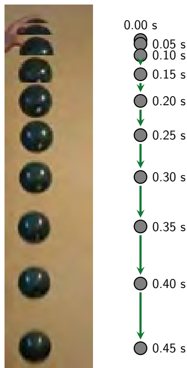
Figure 2.11: Images and corresponding motion map of a falling ball. Images were taken every 0.05 seconds.[1]
