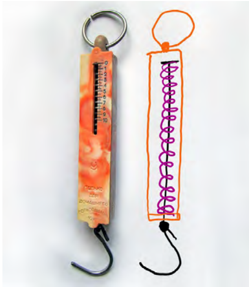
Figure 5.6: A spring scale and a schematic of the way the spring is connected inside.[25]
