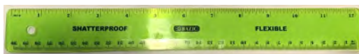
Figure 2.2: Rulers often show inches across the top and centimeters (cm) across the bottom.[1]
