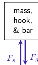
Figure 5.7: FBD of the mass, hook, and metal bar when the system is in equilibrium.[1]
