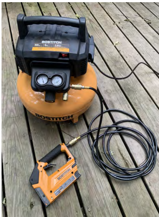
Figure 12.13: Air compressors are designed to hold several atmospheres of air pressure. They are often used for inflating tires and running pneumatic equipment like staplers and nail guns.[1]
