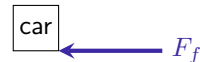
Figure 2.29: FBD of a car that is traveling to the right and braking, horizontal direction only[1]
