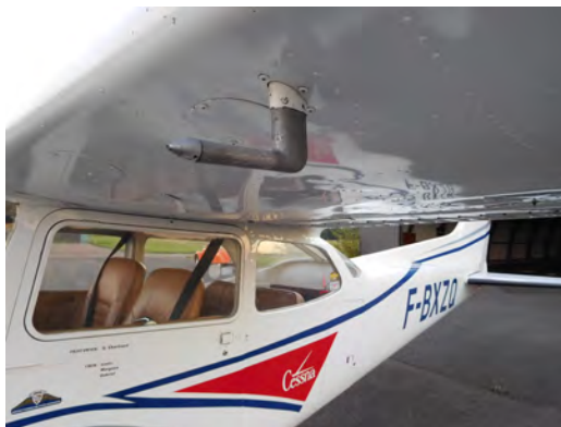
A Pitot tube on the bottom side of an airplane wing.[64]
