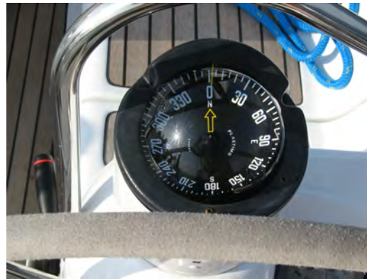
Figure 4.7: Compass bearings start with zero at North and proceed clockwise. Angles in physics usually start at East and proceed counterclockwise.[19]
