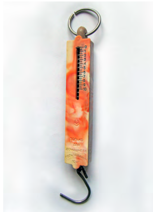
Figure 5.1: A spring scale, which changes in length as the tension force changes.[24]
