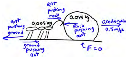
Figure 3.7: A sketch of the ant, the rock, and the forces affecting them. [1]
