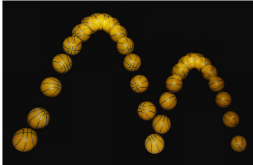
Figure 6.4: This single photograph of a bouncing ball was taken using a stroboscopic light source that flashed 25 times per second .[32]
